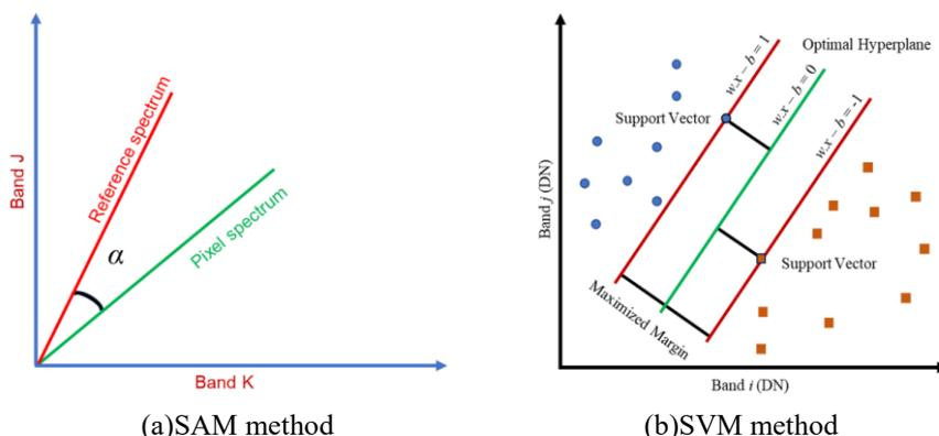
Fig. 3 Schematics of SAM and SVM methods
