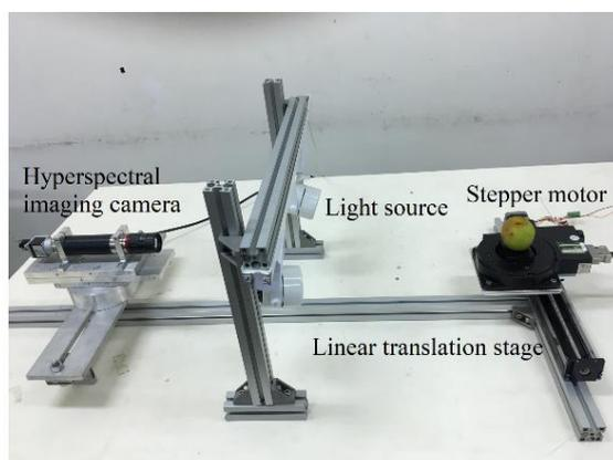
Fig. 2 The design of hyperspectral imaging system
