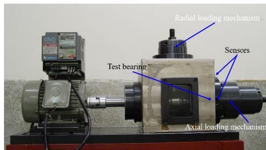
**Fig.1 Schematic of the test rig**
