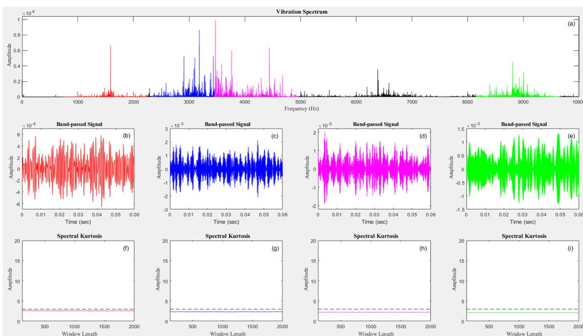
Fig.3 Mean spectral kurtosis analysis for normal bearing running at 1000 rpm
