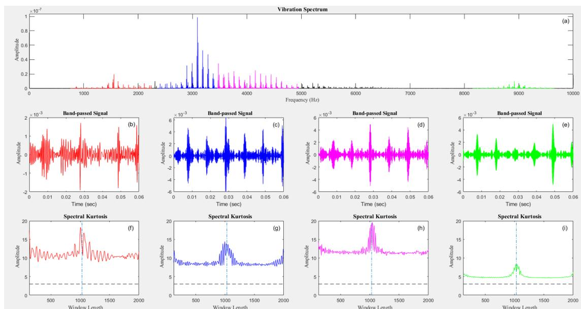
**Fig.2 Mean spectral kurtosis analysis for roller defect bearing running at 1000 rpm**
