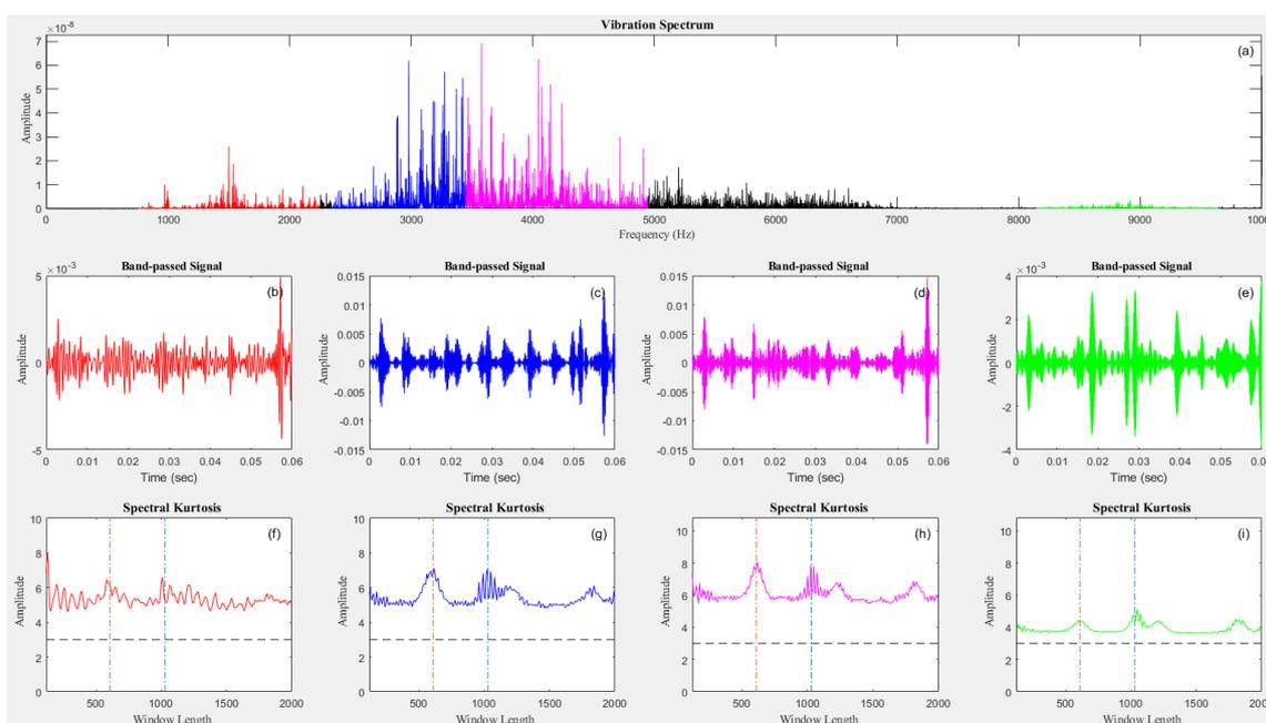
Fig.4 Mean spectral kurtosis analysis for roller and inner-race defect bearing running at 1000 rpm
