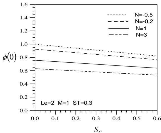
**Fig. 8 Effects of mass stratification parameters on the local surface concentration**
