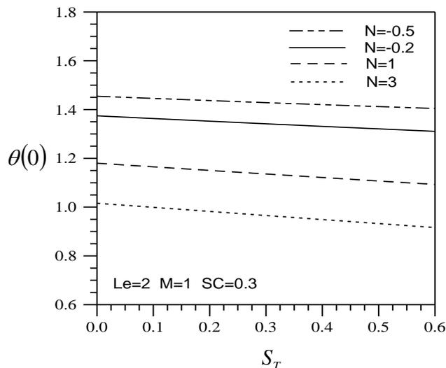
Fig. 6 Effects of thermal stratification parameters on the local surface temperature
