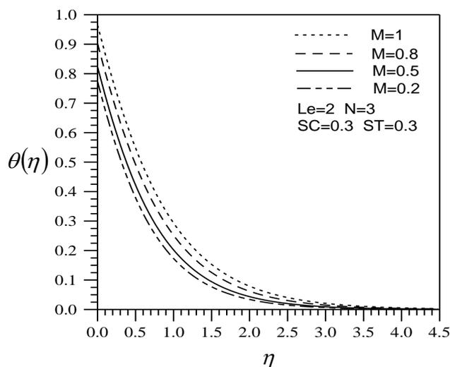
**Fig.2** Effects of magnetic parameters on the temperature profile
