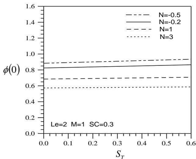
**Fig. 9 Effects of thermal stratification parameters on the local surface concentration**
