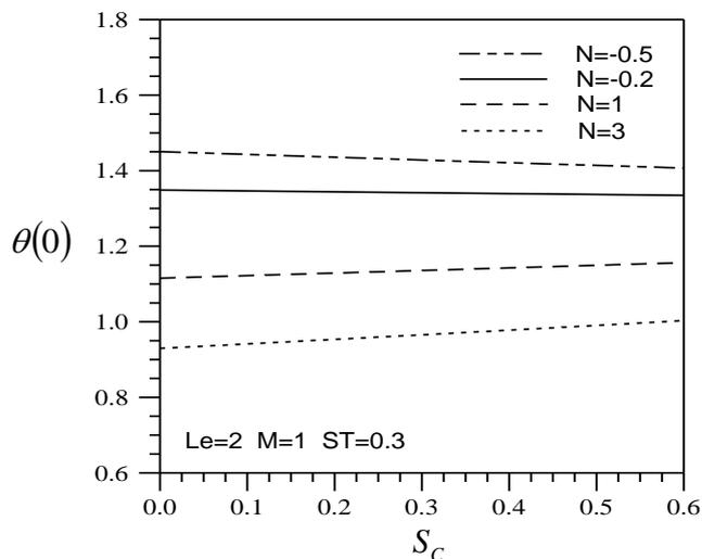
Fig. 7 Effects of mass stratification parameters on the local surface temperature
