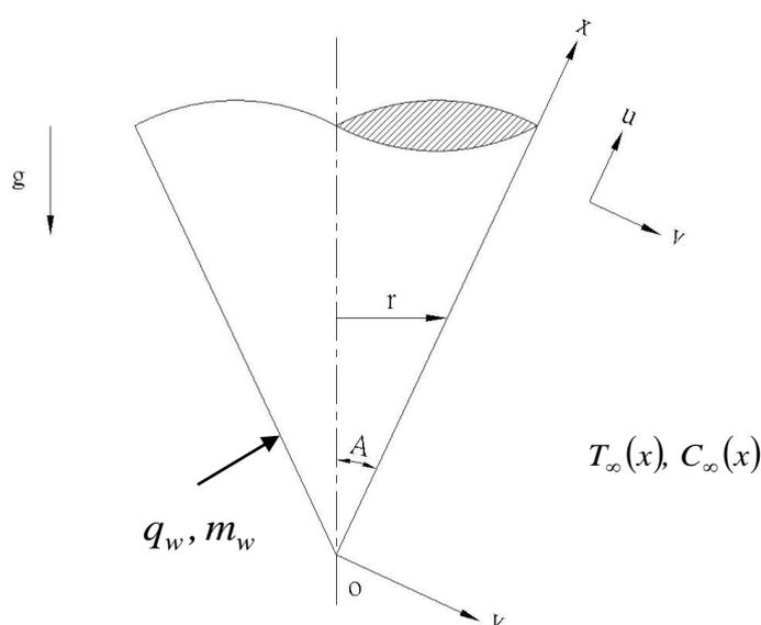
Fig.1 Flow configuration and coordinate system
