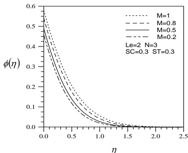
**Fig.3** Effects of magnetic parameters on the concentration profile
